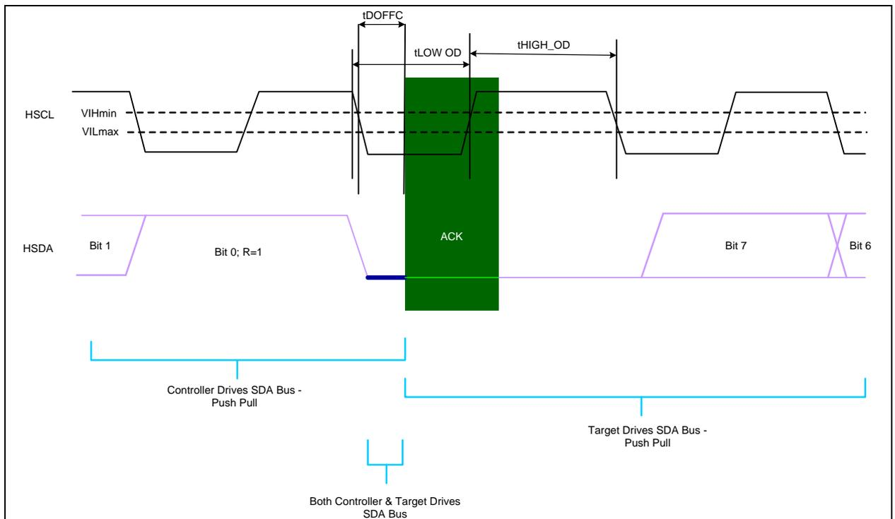
Figure 12. T=1; Host Ends Read with Repeated START and STOP Waveform
