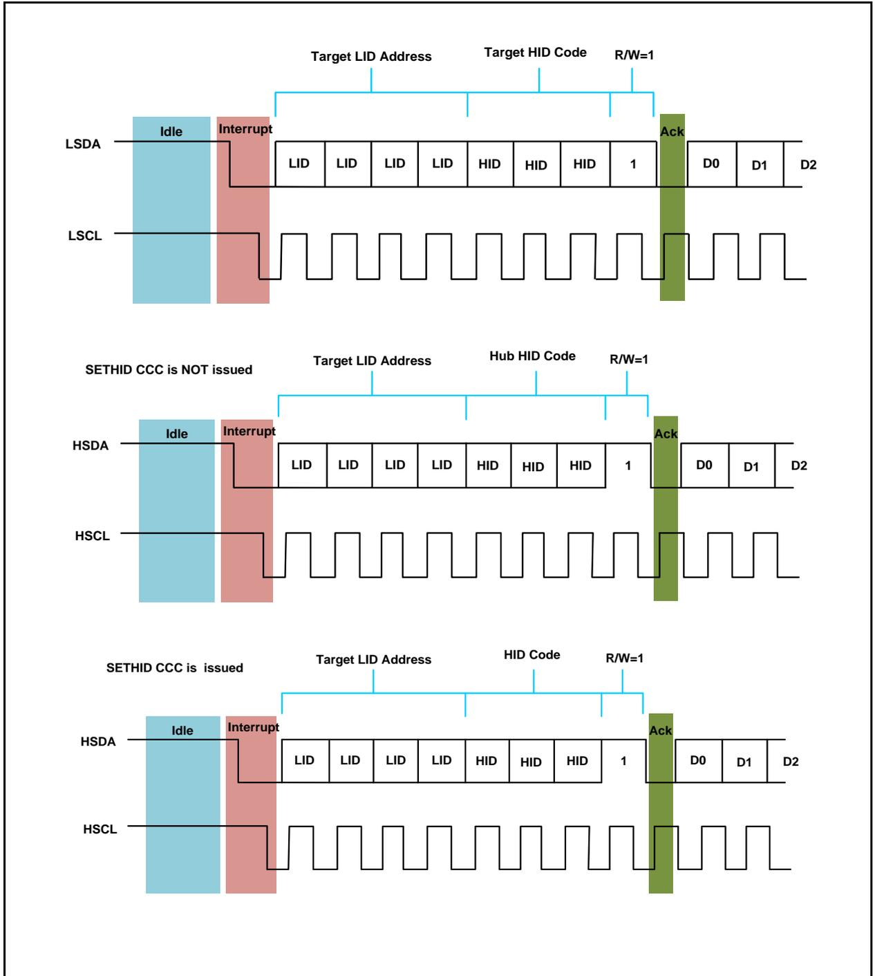
Figure 17. Local Device Interrupt; Host NACK Followed by STOP
