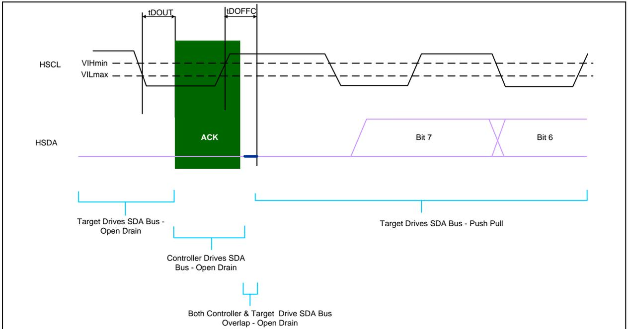
**Figure 11. Controller Push Pull to Target Open Drain Hand Off Operation**
