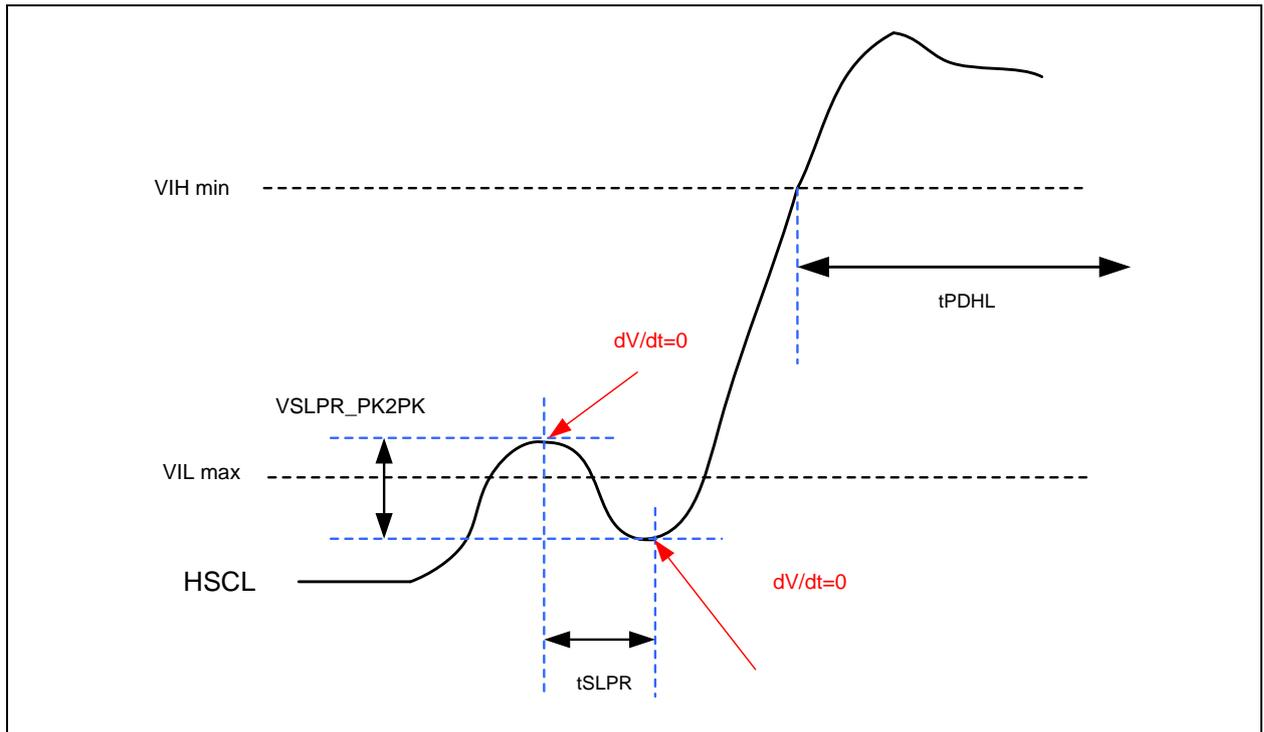
Note that  $t_{PDHL}$  is for reference only in this diagram, refer to measurement methodology for details on this parameter.
