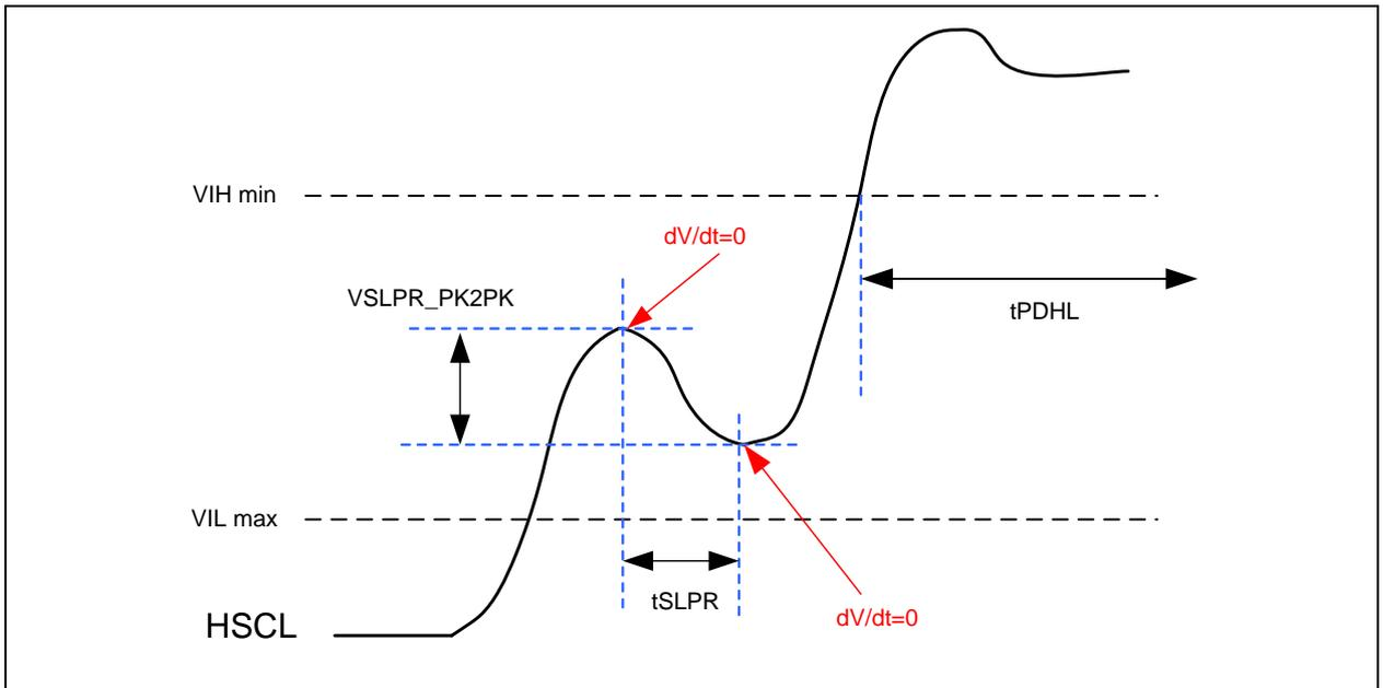
Note that  $t_{PDHL}$  is for reference only in this diagram, refer to measurement methodology for details on this parameter.
