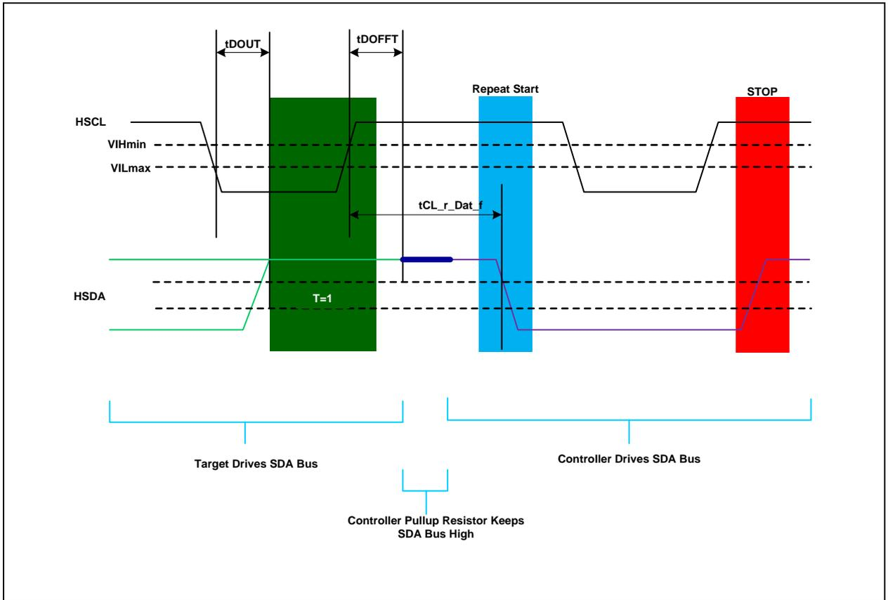
Figure 13. T=0; Target Ends Read; Host Generates STOP
