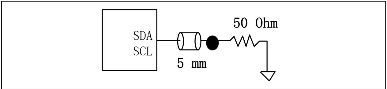
Figure 23. Output Slew Rate Measurement Points
