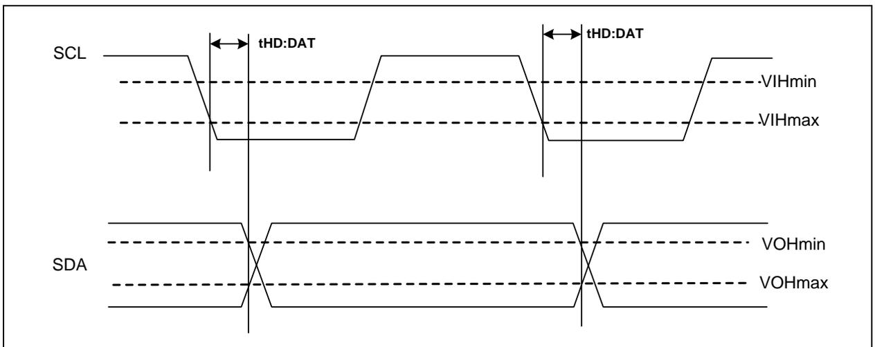
Figure 22. Output Slew Rate and Output Timing Reference Load
