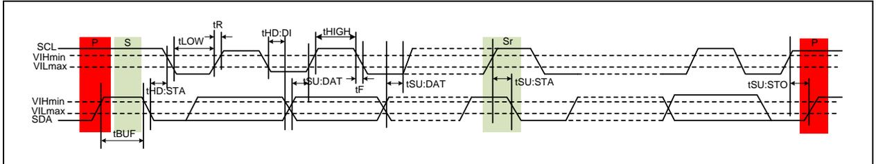
**Figure 20. I3C Basic Bus AC Data Output Timing Parameter Definition**
