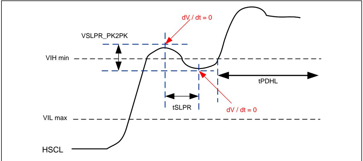
Note that  $t_{PDHL}$  is for reference only in this diagram, refer to measurement methodology for details on this parameter.
