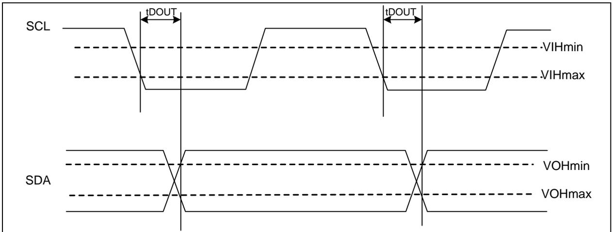
**Figure 21. I<sup>2</sup>C Bus AC Data Output Timing Parameter Definition**
