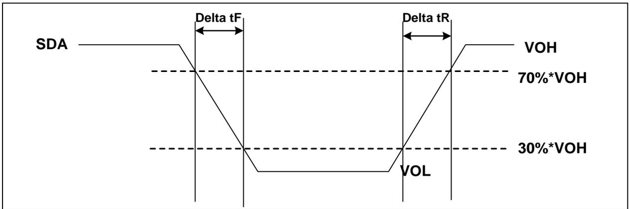
Figure 24. Rise and Fall Timing Parameter Definition
