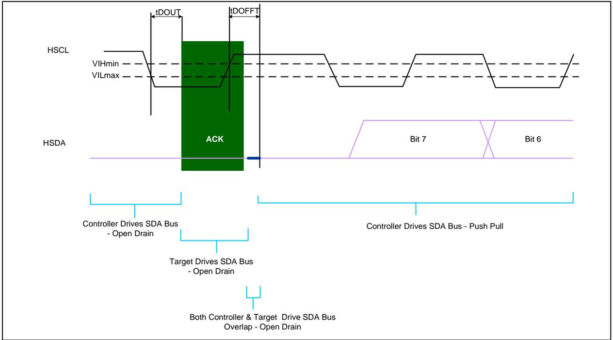
**Figure 10. Controller Open Drain (ACK) to Target Push Pull Hand Off Operation**
